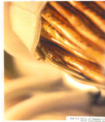
Faulty wiring that led to Titan 4A failure
